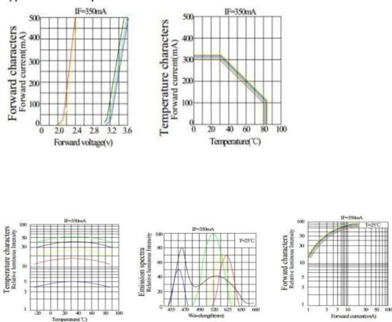
Typical electrical-optical Characteristics curvers
